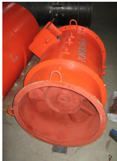
Figure 4: New axial ventilation fan
