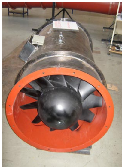
Figure 5: Existing steel axial ventilation fan
